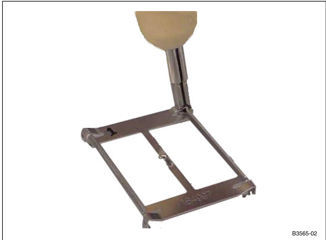
Figure 12. Hand-Tool on Heat-Sink Clip Assembly
