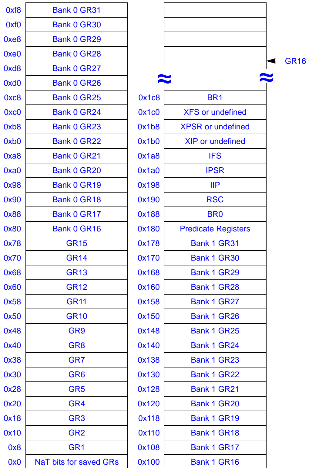
Figure 11-14. Processor State Saved in Min-state Save Area
