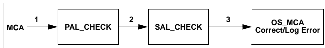
Figure 13-4. Uncorrectable Machine Check Code Flow
