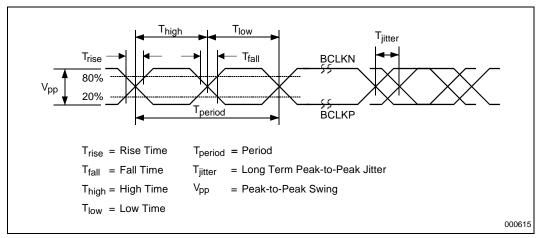
Figure 2-2. SMSC Clock Waveform
