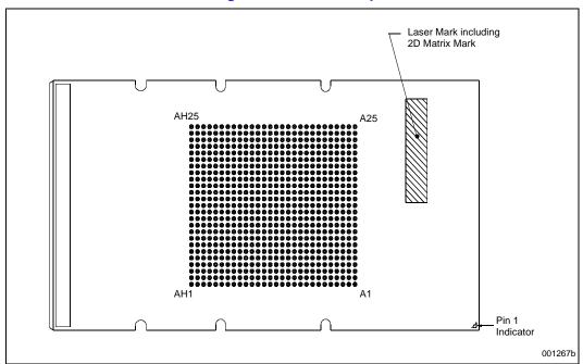
Figure 4-5. Processor Bottom-Side Marking Placement on Interposer
