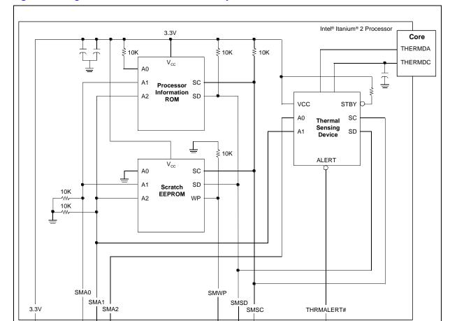
Figure 6-1. Logical Schematic of SMBus Circuitry
