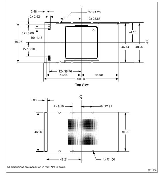
Figure 4-3. Itanium<sup>®</sup> 2 Processor Package Power Tab
