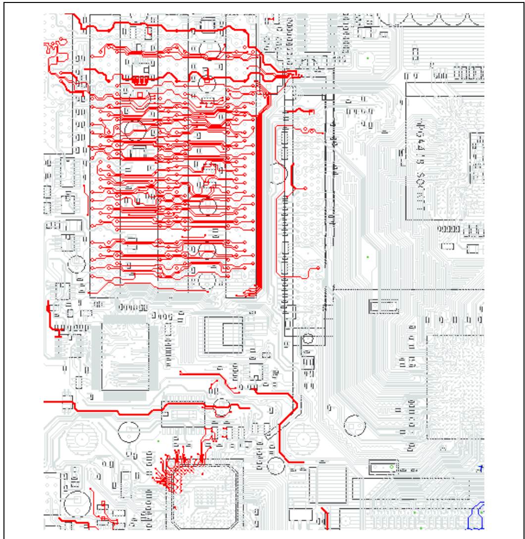
Figure 111. Example PCI Routing on Layer 1
