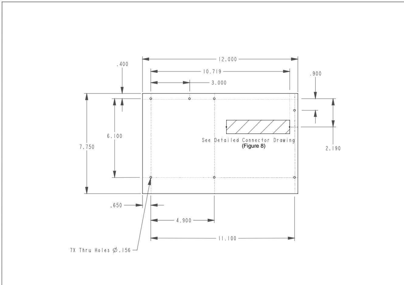
**Figure 14: ATX Motherboard Layout Details**
