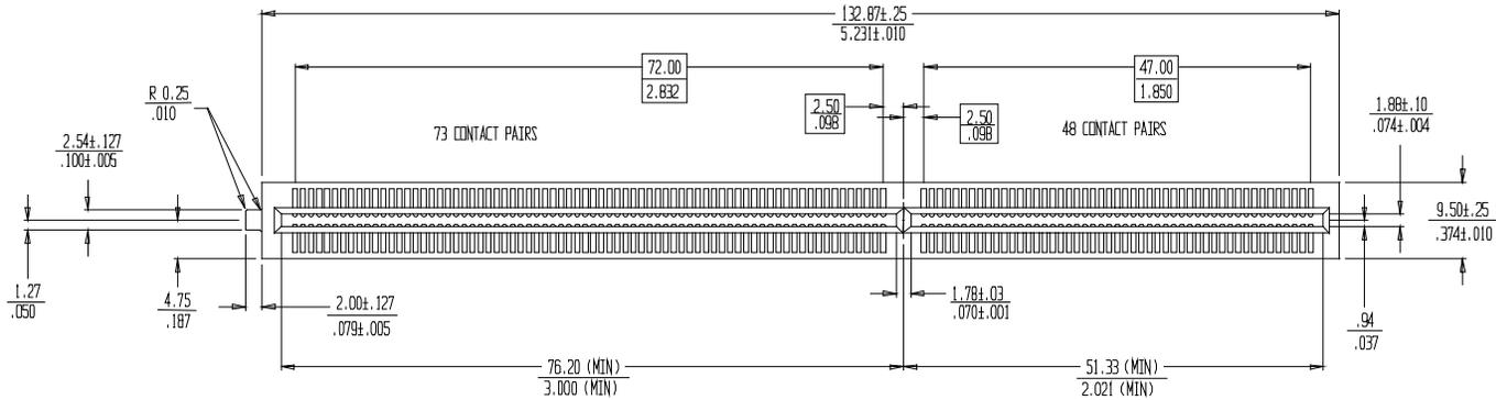
Figure 5: Connector Dimensions, con't.
