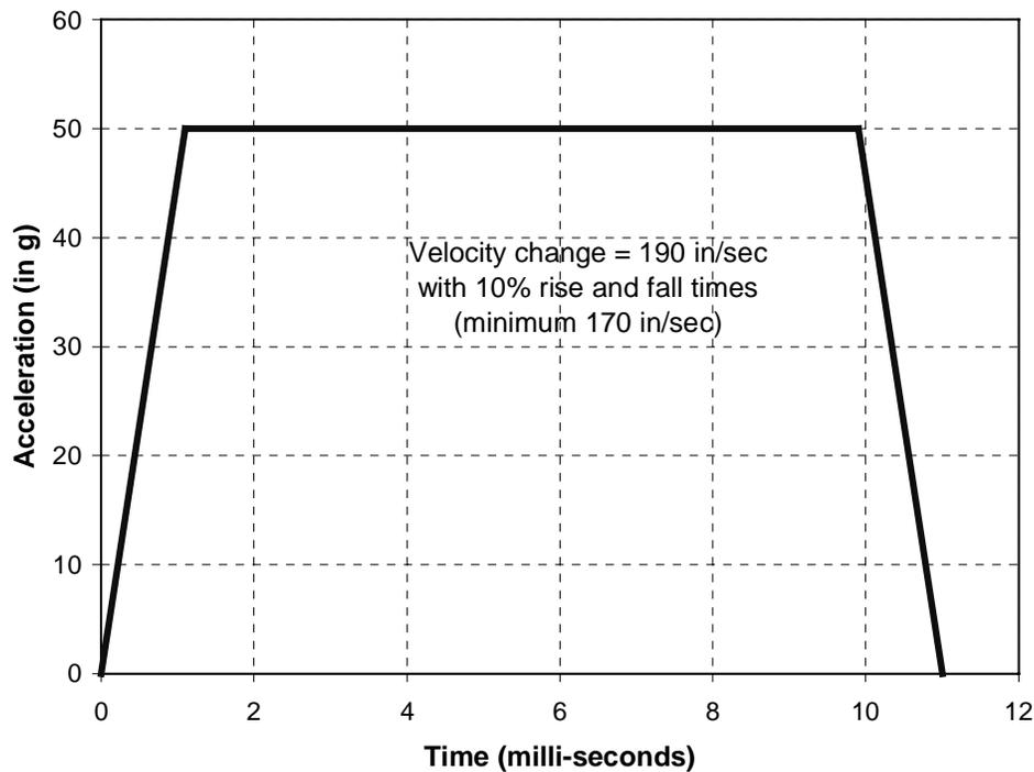
**Figure 15: Shock Pulse Curve**
