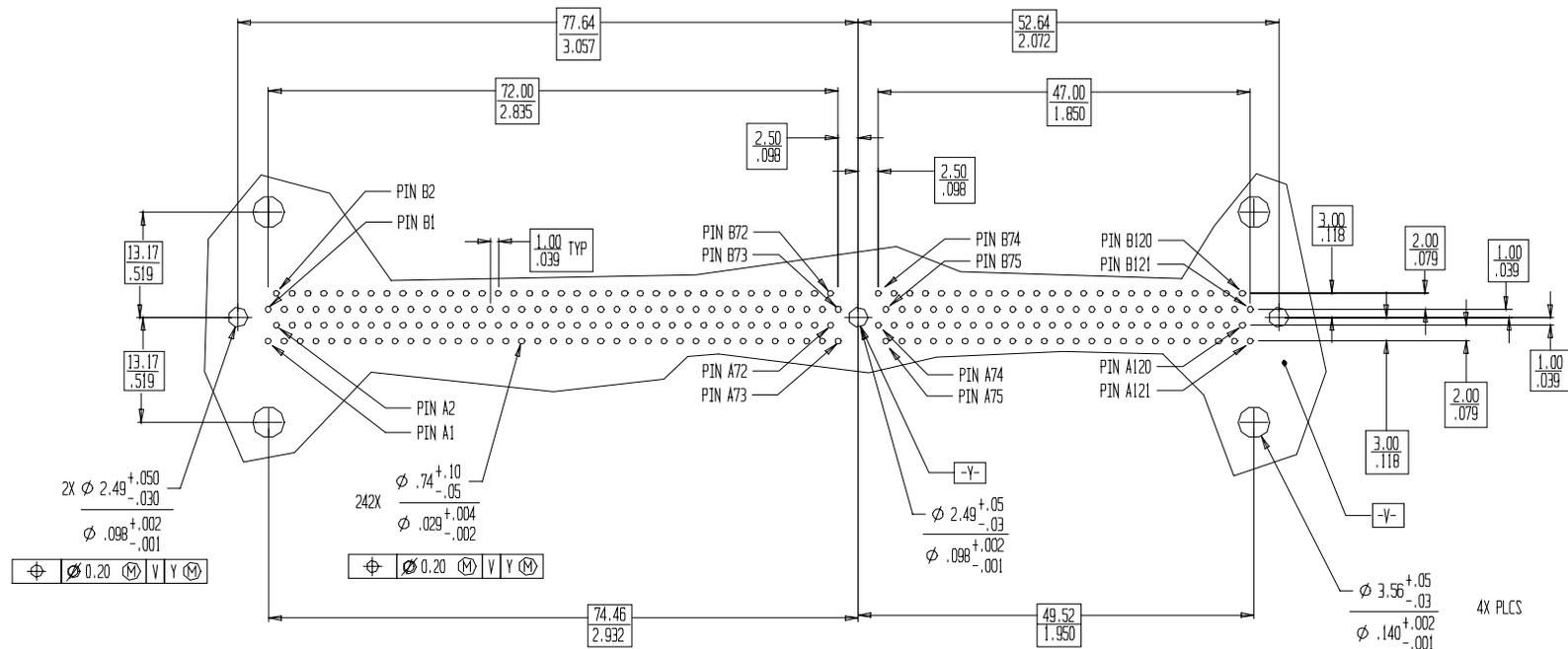
**Recommended clearances around 3.56 mm DIA (0.140 inch DIA) mounting Holes:**
