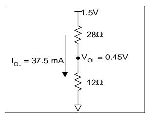
Figure 4. Equivalent circuit for output low state.
