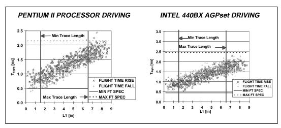
Figure 19. Monte Carlo flight times for single processor design
