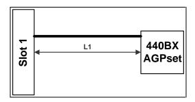
Figure 23. Topology for single processor designs with single end termination (SET)
