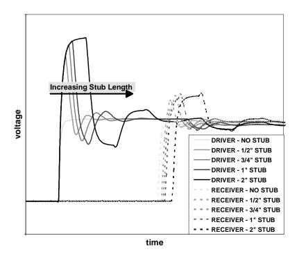
Figure 7. Ringing as a function of stub length for the network in Figure 3.
