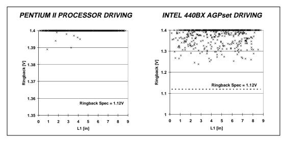
Figure 20. Monte Carlo signal quality for single processor design
