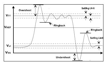
Figure 14. Overshoot, ringback, and settling time
