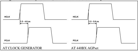
Figure 25. Host-to-PCI clock lag spec
