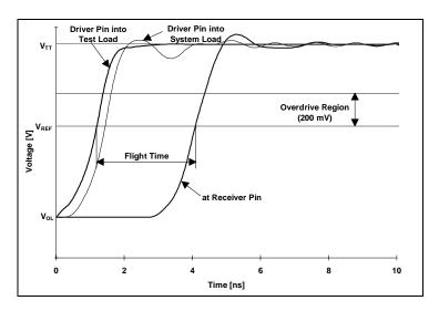
Figure 10. Nominal flight time measurement
