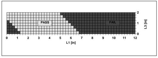
Figure 18. Solution space for single processor design, based on results of parametric sweeps
