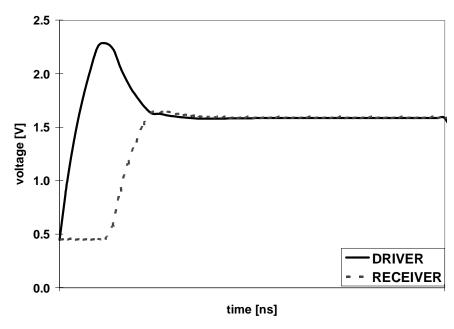
Figure 9. Waveform for the network in Figure 3 when driven with active pull-up
