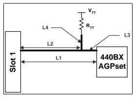
Figure 15. Recommended topology for single processor design
