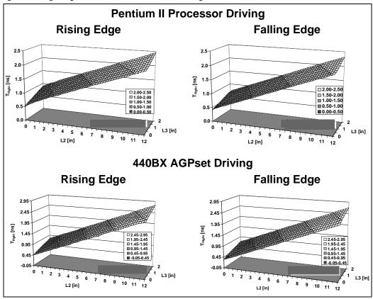
Figure 16. Parametric sweep minimum flight times for single processor design
