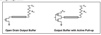
Figure 8. GTL+ buffer types - open drain and active pull-up
