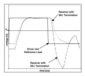
Figure 2. GTL+ flight time dependence on R<sub>TT</sub>.
