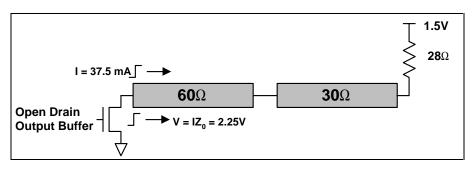
Figure 5. Waveform launch for low-high signal transition.
