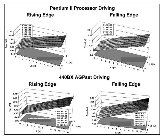
Figure 17. Parametric sweep maximum flight times for single processor design
