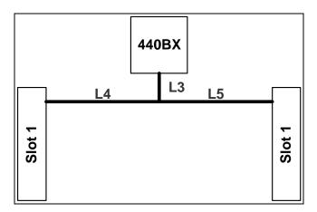
Figure 21. Recommended topology for dual processor design
