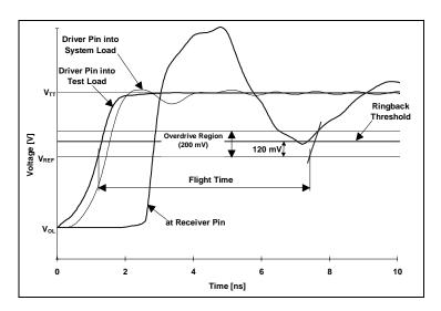
Figure 12. Flight time measurement with non-monotonic rising edge
