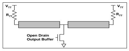
Figure 1. GTL+ open drain buffer with external pull-up to  $V_{\rm TT}$ .
