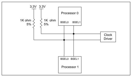
Figure 5. Differential Clock BSEL Circuit
