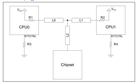
Note: R3 and R4 determine the nominal values of R1 and R2, respectively. Please refer to the LV Intel® Pentium® III Processor 512K Dual Processor Platform Design Guide for further dual processor system bus layout and topology information.
