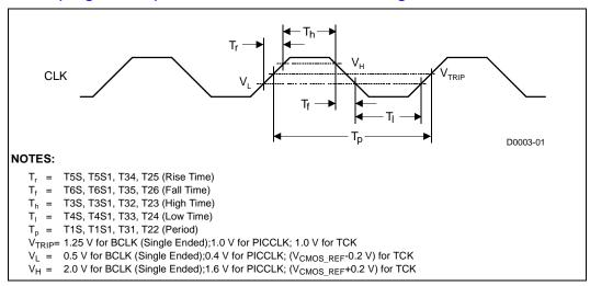
Figure 11. Differential BCLK/BCLK# Waveform (Common Mode)
