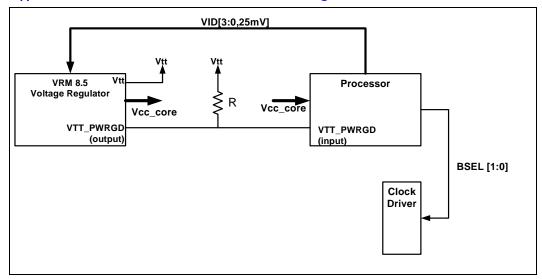
*Note:* Please refer to the *LV Intel*<sup>®</sup> *Pentium*<sup>®</sup> *III Processor 512K Dual Processor Platform Design Guide* for VTT\_PWRGD implementation for an LV Intel Pentium III processor 512K platform.
