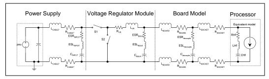
Figure 5-3. Detailed Power Distribution Model for System with VRM
