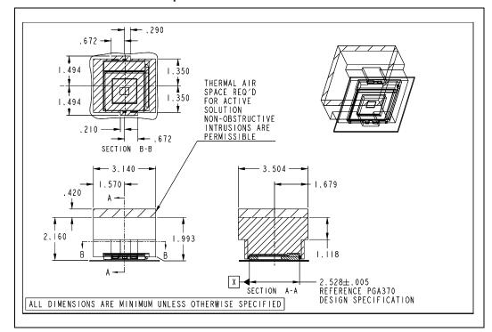
Figure 2-3. Socket 370 Volumetric Keepout
