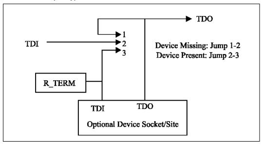
Figure 3-10. 4-Pin Jumper Bypass
