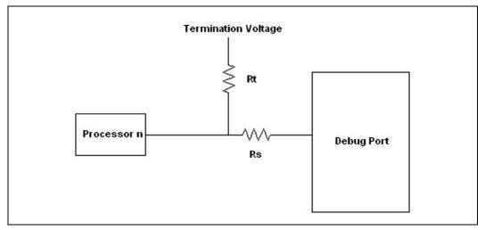
Figure 3-7. RESET# Signal Termination
