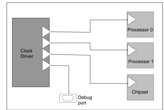
Figure 4-1. Host Bus Clock Connections
