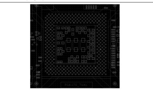
Figure 5-6. PGA370 Decoupling Capacitor Placement
