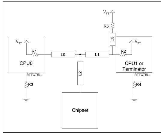
Figure 3-2. Terminator-less System Bus T Topology
