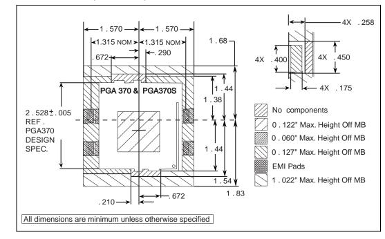
Figure 2-2. Socket 370 Component Keepout
