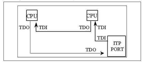
Figure 3-9. TDO 3-Pin Jumper Bypass
