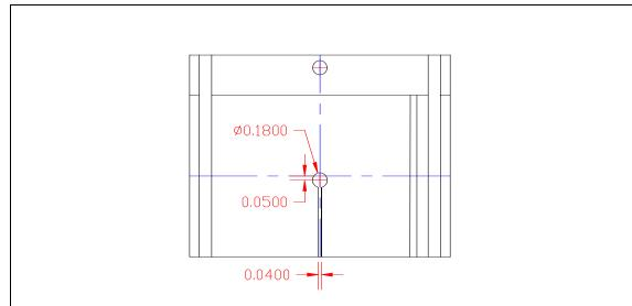
Figure 7-8. Example of Dimensioning for Thermocouple Groove
