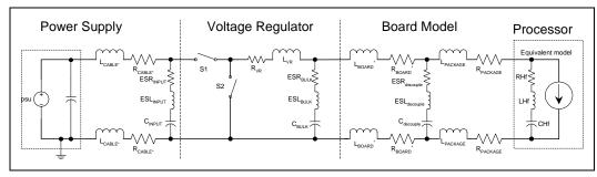
The voltage regulator should be designed in conjunction with the recommended load model referenced in Figure 19.
