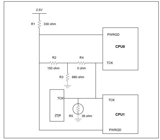
Figure 23. LV Intel Pentium III processor 512K Example THERMTRIP# Workaround Circuit
