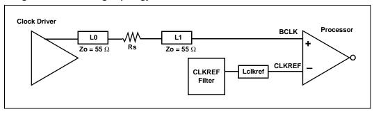
Figure 13 shows the topology that should be used for the chipset clock traces. Note that Ln refers to trace lengths between the illustrated components. Table 15 contains the recommended lengths and component values for this topology.
