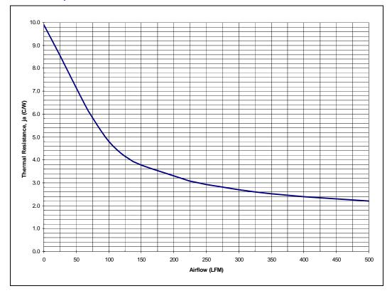
Figure 5. Heat Sink Option 1 Thermal Performance Curve
