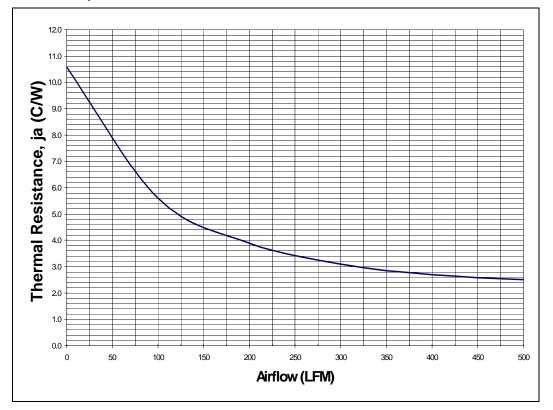
Figure 8. Heat Sink Option 2 Thermal Performance Curve
