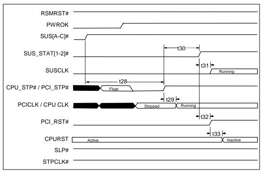
Table 41. Mechanical Off to On Timing
