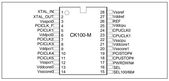
Figure 10. Pinout for CKBF-M Compatible Clock Buffer
