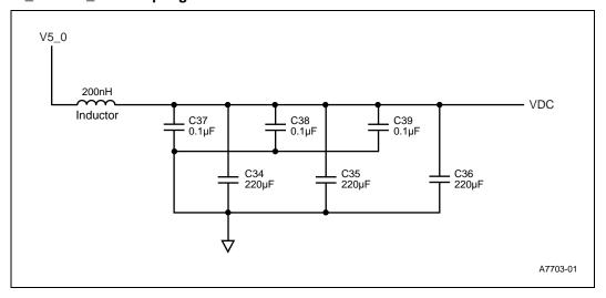
Exact component values are system dependant. Intel recommends that specific component values be determined through full simulation and parasitic modeling.
