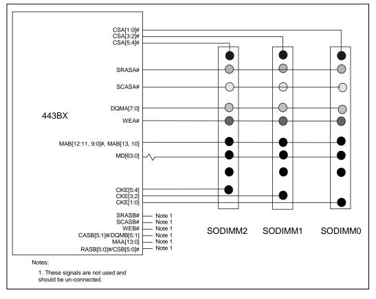
Figure 7. SDRAM - Three SODIMMs
