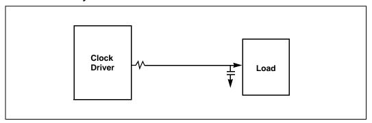
This optional layout implementation is suggested to accommodate clock tuning, HCLK & PCICLK from CK100-M and SCLK from CKBF-M. This will allow the designer to tune the individual clock signals to minimize EMI and allow for variations in impedance, skew and loading.
