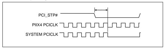
Figure 24 describes the timing requirements for the control of the system PCICLK. The system PCICLK timings shown Figure 24 must be followed exactly for proper operation of PC/PCI DMA or Serial IRQ logic. When PC/PCI DMA and Serial IRQs are not used in the system, the system PCICLK stop timings must meet the system developer's requirements.
