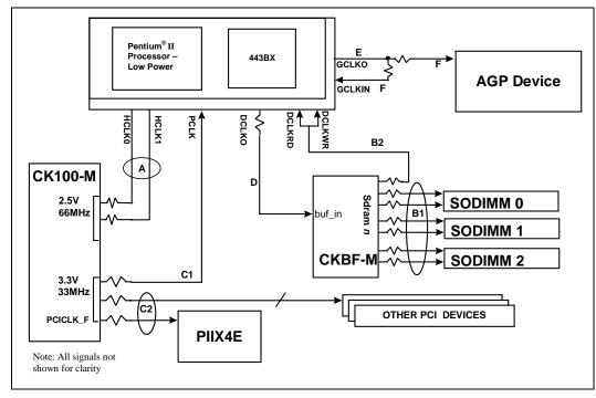
Figure 12. Low-Power Module Clocking Layout
