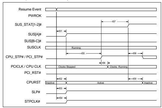
Table 44. POS to On (with Processor Reset) Timing
