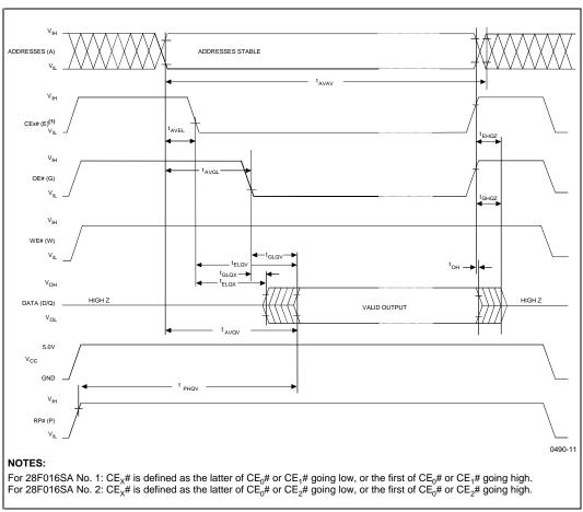
Figure 11. Read Timing Waveforms
