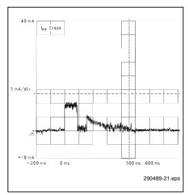
Figure 20. I<sub>PP</sub> during Block Erase
