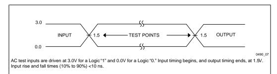
Figure 7. Transient Input/Output Reference Waveform (V<sub>CC</sub> = 3.3V) and High Speed Reference Waveform  $^{(2)}$  (V<sub>CC</sub> = 5.0V  $\pm$  5%)
