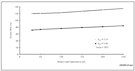
Figure 21. Access Time  $(t_{ACC})$  vs. Output Loading
