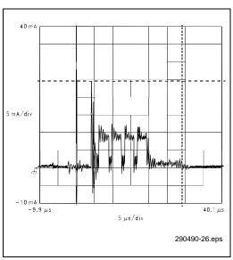
Figure 23. I<sub>PP</sub> during Page Buffer Write Operation
