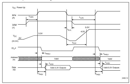
Figure 13.  $V_{CC}$  Power-Up and RP# Reset Waveforms
