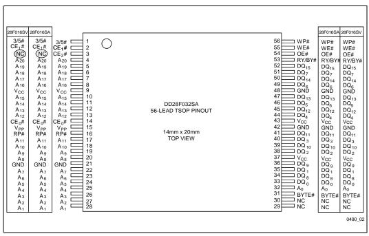
Figure 2. Dual Die TSOP Pinout Configuration
