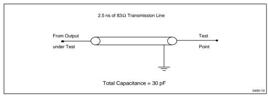
Figure 10. High Speed Transient Equivalent Testing Load Circuit ( $V_{CC} = 5.0V \pm 5\%$ )
