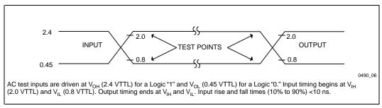
Figure 6. Transient Input/Output Reference Waveform (V<sub>CC</sub> = 5.0V) for Standard Test Configuration<sup>(1)</sup>
