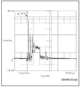
Figure 22. I<sub>PP</sub> during Word Write Operation
