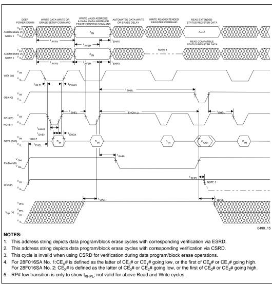
Figure 15. Alternate AC Waveforms for Command Write Operations
