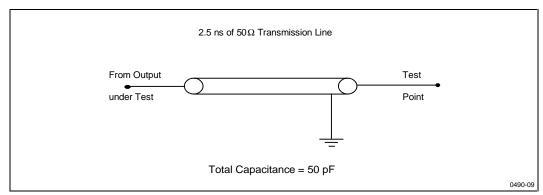
Figure 9. Transient Equivalent Testing Load Circuit ( $V_{CC} = 3.3V \pm 0.3V$ )
