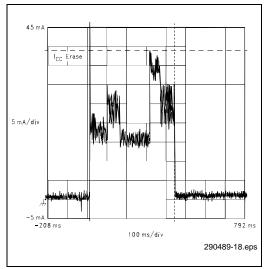
Figure 18. I<sub>CC</sub> during Block Erase
