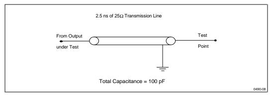
Figure 8. Transient Equivalent Testing Load Circuit ( $V_{CC} = 5.0V \pm 10\%$ )
