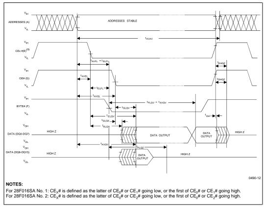
Figure 12. BYTE# Timing Waveforms
