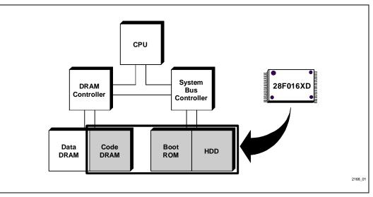
Figure 1. The 28F016XD Eliminates the Need to Shadow Code from a Slow, Nonvolatile Memory Source to a Faster, Volatile Execution Memory
