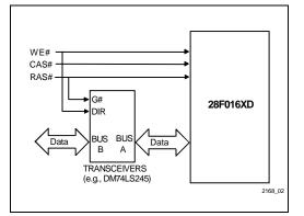
Figure 2. 28F016XD-Data Path Transceivers Eliminate Potential Bus Contention Issues
