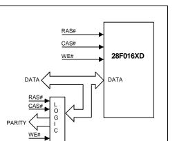
Figure 4. Simple Logic Can Implement Parity Generation for 28F016XD-Based Memory Banks
