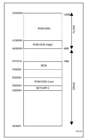
Figure 6. Intel486 Microprocessor System Memory Map with 28F016XD SIMM
