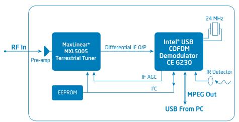
The Intel CE 9500 reference design includes all necessary support features and functions including DC-DC conversion, active-antenna support and an on-board remote control IR interface. The receiver is designed to meet NorDig Unified RF field requirements, USB 2.0 and EMC standards. The design includes a complete set of design and manufacturing support collateral to enable you to accelerate time-to-market for a DVB-T PC-TV USB stick product.
