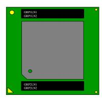
$\label{eq:GRP1LN1:INTEL} $$ GRP1LN1: INTEL (m)(c) '01_-_{Country of Origin} $$ GRP1LN2: {Core freq}/{Cache}/{Bus Freq}/{Voltage}$$$
