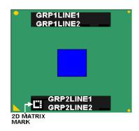
$\label{eq:grp1LN1:INTEL} $$ GRP1LN1: INTEL (m)(c) '01_-_{COO} $$ GRP1LN2: {Core Freq}/{Cache}/{Bus Freq}/{Voltage} $$$
