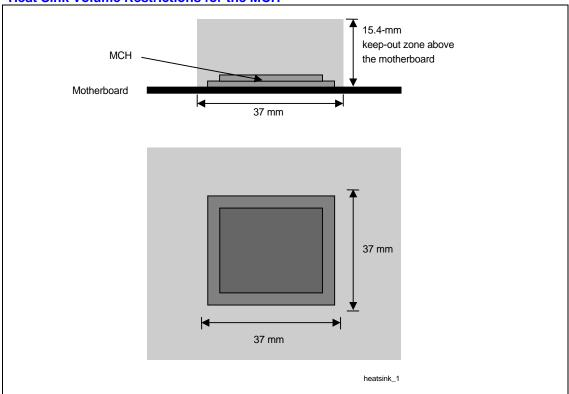
Figure 7. Heat Sink Volume Restrictions for the MCH
