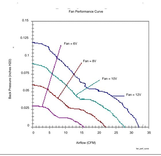
The use of multiple (identical) fans in a system does provide marginally increased airflow. The exact amount depends on many factors, including the fan speed and configuration as well as the chassis airflow impedance. If the fans are not identical, then the figures will change slightly, but the trends will be the similar. The general rules are as follows: If the chassis has high system impedance, place the fans in series. If the chassis has low system impedance, place the fans in parallel.
