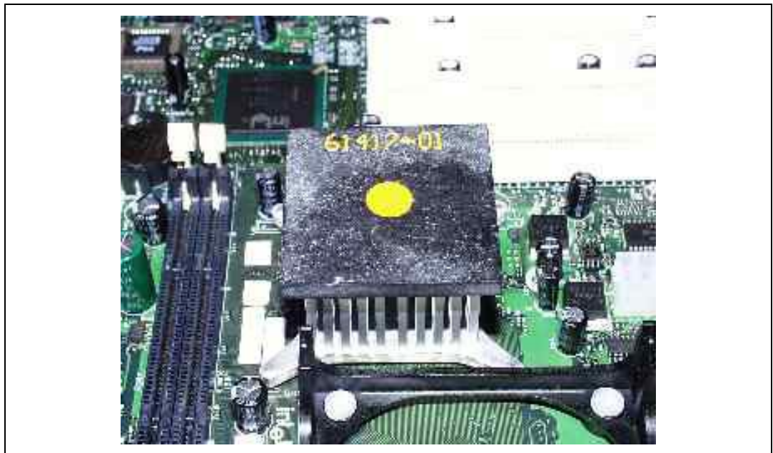
Figure 14. WSHS Target (Heatsink Shown Is Not (G)MCH WSHS)
