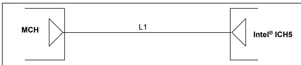
Figure 7-2. Hub Interface Signal Routing Topology
