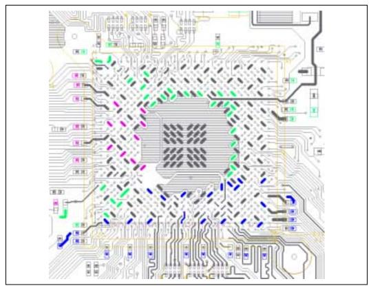
Figure 43. Intel® 815P Chipset Platform Decoupling Example
