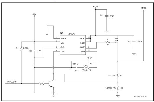
Figure 49. AGP VDDQ Generation Example Circuit
