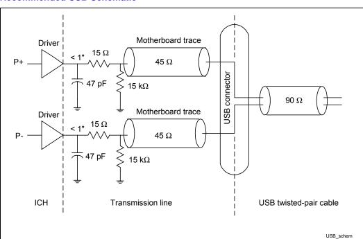
Figure 61. Recommended USB Schematic
