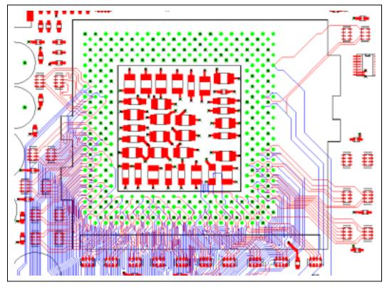
Figure 31. Capacitor Placement on the Motherboard
