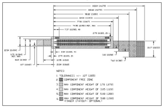
Figure 45. AGP Left-Handed Retention Mechanism Keep-Out Information
