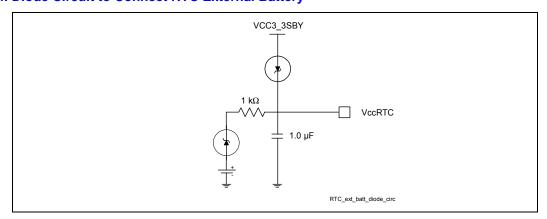
A standby power supply should be used to provide continuous power to the RTC when available, which will significantly increase the RTC battery life and thereby the RTC accuracy.
