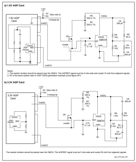
The flexible VREF divider shown in Figure 50 uses a FET switch to switch between the locally generated VREF (for 3.3 V add-in cards) and the source-generated VREF (for 1.5 V add-in cards).
