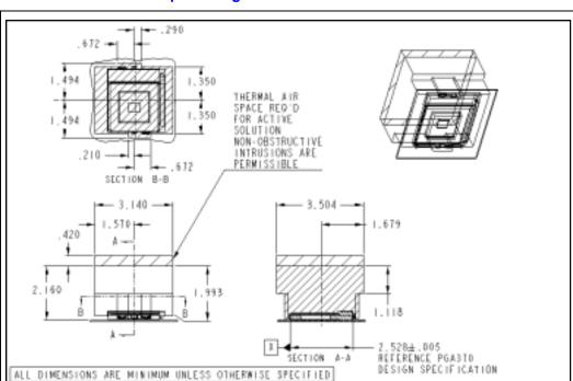
Figure 32. Heatsink Volumetric Keep-Out Regions
