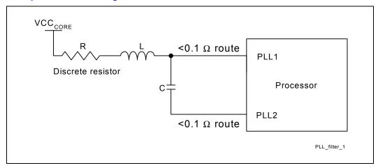
Figure 29. Example PLL Filter Using a Buried Resistor
