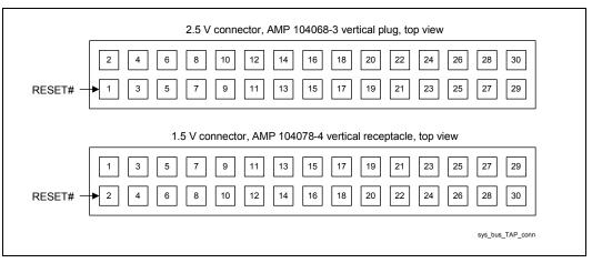
Caution: Pentium III processor (CPUID=068xh) and Celeron processor (CPUID=068xh) require an intarget probe (ITP) compatible with 1.5 V signal levels on the TAP. Previous ITPs were designed to work with higher voltages and may damage the processor if connected to any of these specified processors.
