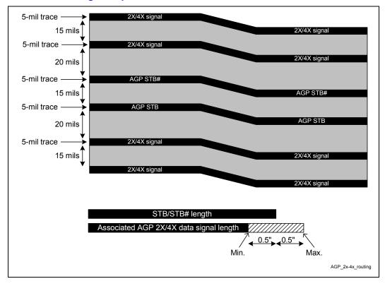
Figure 46. AGP 2X/4X Routing Example for Interfaces < 6 Inches and GPA/AGP Solutions
