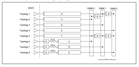
In addition to meeting the spacing requirements outlined in Table 20, system memory signal trace edges must be at least 30 mils from any other non-system memory signal trace edge.
