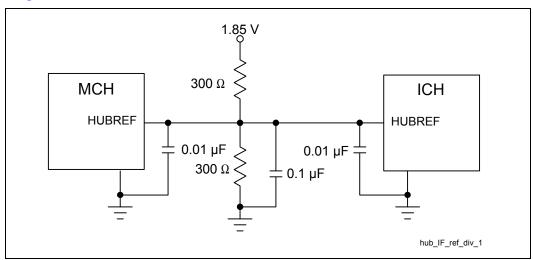
Figure 52. Single-Hub-Interface Reference Divider Circuit
