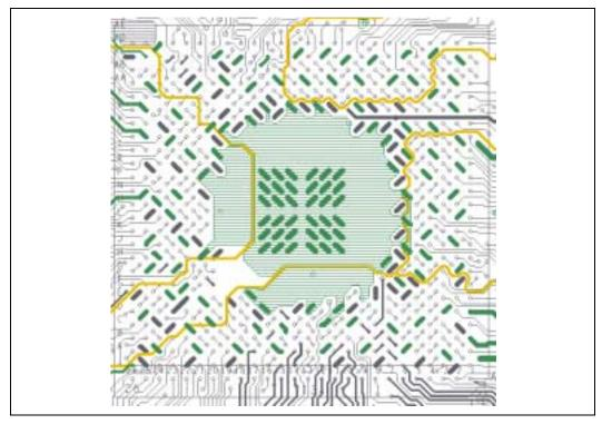
Figure 42. Intel® 815P Chipset Platform Decoupling Example
