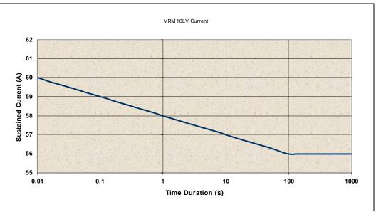
**NOTES:** 1. Processor or voltage regulator thermal protection circuitry should not trip for load currents greater than I<sub>CC\_TDC</sub>. 2. Not 100% tested. Specified by design characterization.
