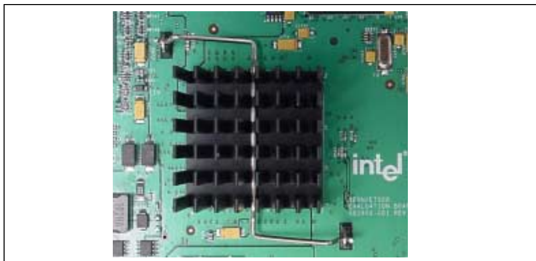
Figure 5. Installed MCH Heatsink
