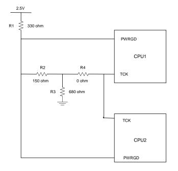
Assumes the inputs to the CPU\_PWRGD are open collector signals that are Wire-ANDed together
