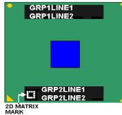
GRP1LN1: INTEL (m)(c) '01\_-\_{COO} GRP1LN2: {Speed}/{Cache}/{Bus}/{Voltage}
