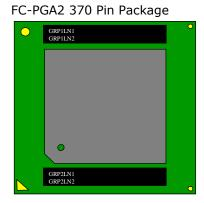
GRP1LN1: INTEL (m)(c) '01\_-\_{Country of Origin} GRP1LN2: {Core freq}/{Cache}/{Bus Freq}/{Voltage}
