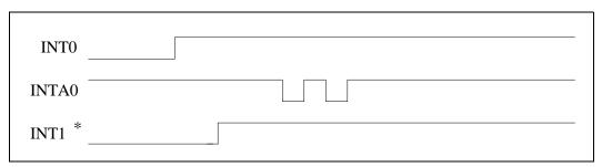
Figure 4. Correct INT0 Acknowledge Operation with a Simultaneous INT1
