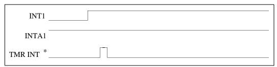
Figure 2. Incorrect INT1 Acknowledge Sequence with Higher Priority Timer Interrupt
