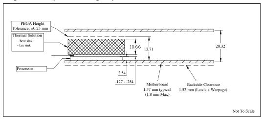
Figure 3. Double-Slot CompactPCI Z-Height Specification
