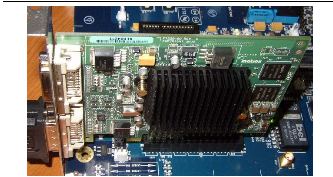
Figure 23. Graphics Adapter Installation - PCIe Slot 0
