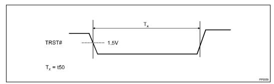
Figure 9. Test Reset Timings
