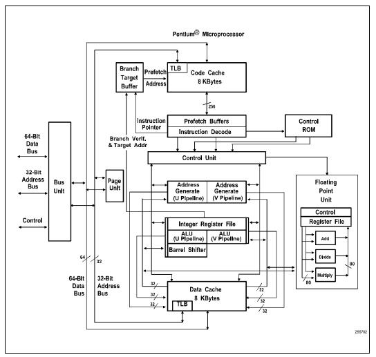
Figure 1. Pentium ® Processor Block Diagram
