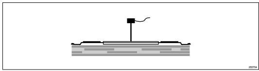
Figure 20. Technique for Measuring Case Temperature (T  $_{
