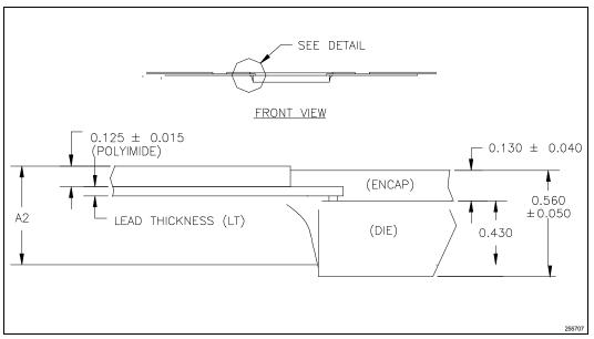
Figure 18. One TCP Site (Cross-Sectional Detail)
