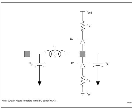
Figure 10. Input Buffer Model, Except Special Group
