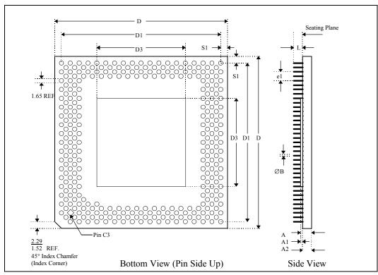
Figure 22. 296-Pin Ceramic Pin Grid Array Package
