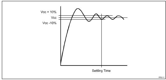
Figure 14. Settling Time
