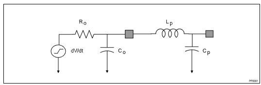
Figure 12. First Order Output Buffer Model
