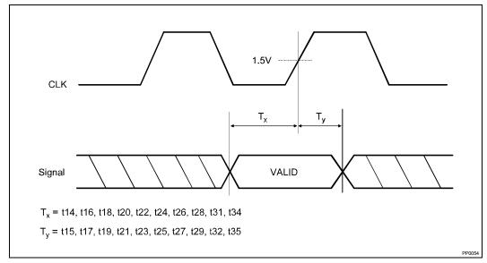
Figure 6. Setup and Hold Timings
