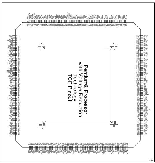
Figure 2. TCP Pentium ® Processor Pinout
