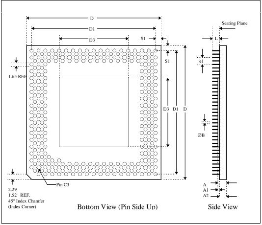
Figure 22. 296-Pin Ceramic Pin Grid Array Package
