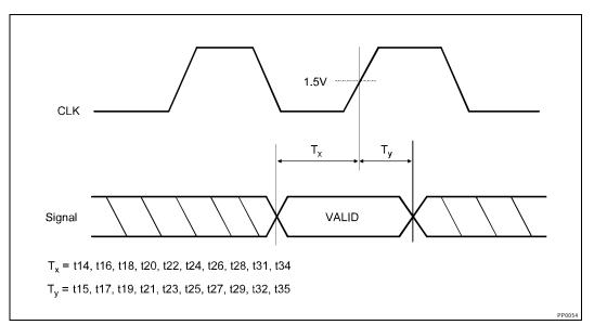
Figure 6. Setup and Hold Timings
