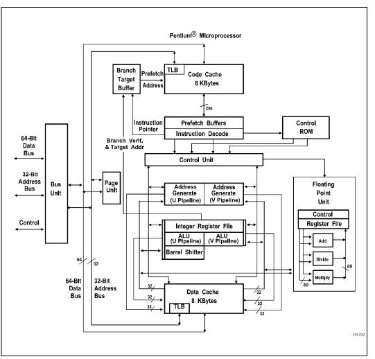
Figure 1. Pentium® Processor Block Diagram
