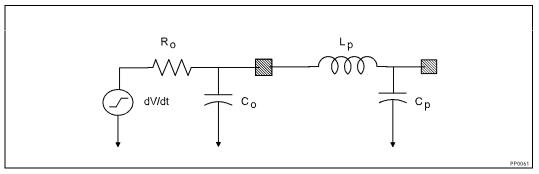
Figure 12. First Order Output Buffer Model
