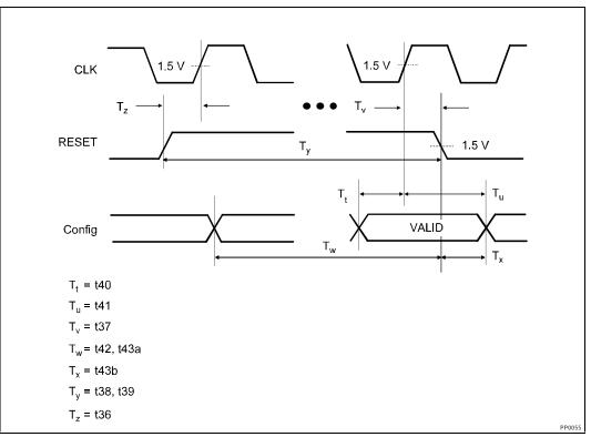
Figure 7. Reset and Configuration Timings
