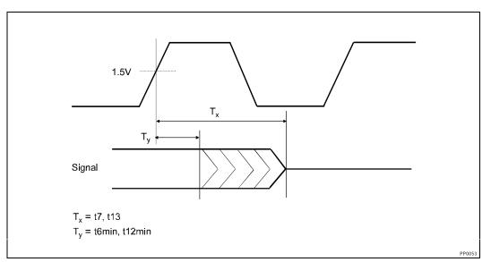
Figure 5. Float Delay Timings
