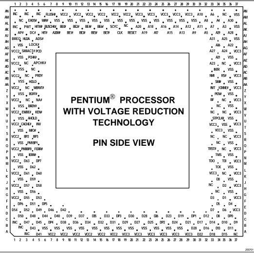
Figure 21. SPGA Pentium<sup>®</sup> Processor with Voltage Reduction Technology Pinout
