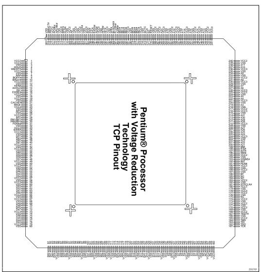
Figure 2. TCP Pentium® Processor Pinout
