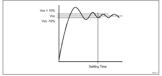
Figure 14. Settling Time
