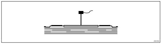
Figure 20. Technique for Measuring Case Temperature (T<sub>C</sub>)
