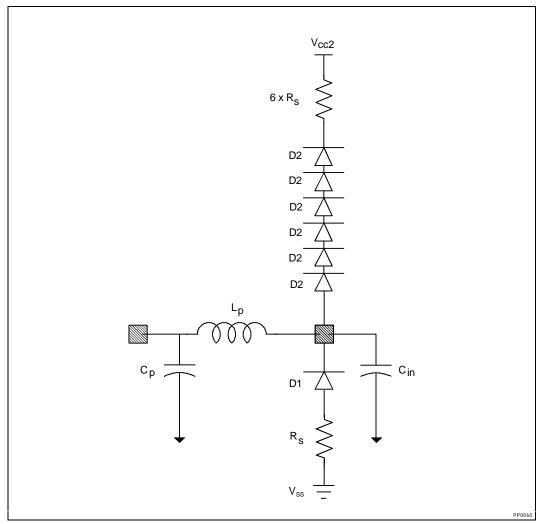
Figure 11. Input Buffer Model for Special Group
