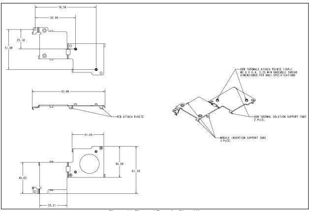
Figure 14. Thermal Transfer Plate (A)
