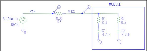
Figure 6. Instantaneous In-rush Current Model
