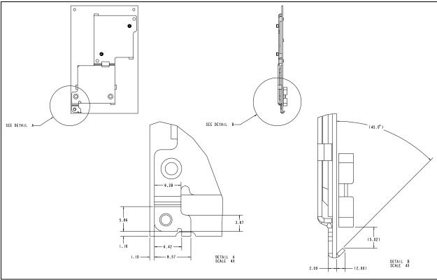
Figure 15. Thermal Transfer Plate (B)
