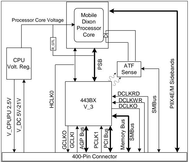
Figure 1 illustrates the block diagram of the Pentium II processor with on-die cache mobile module MMC-2.
