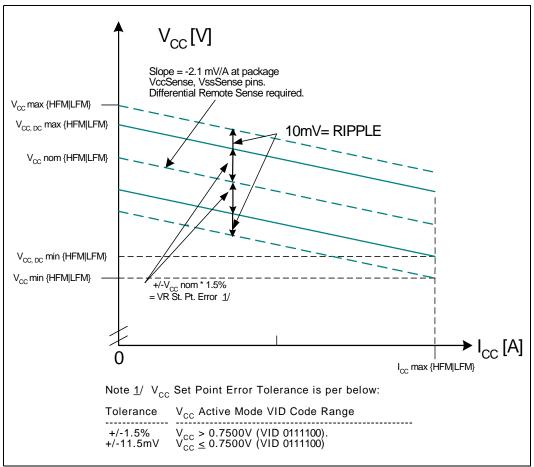
NOTE: For low voltage, if PSI# is not asserted then the 13-mV ripple allowance becomes 10 mV.
