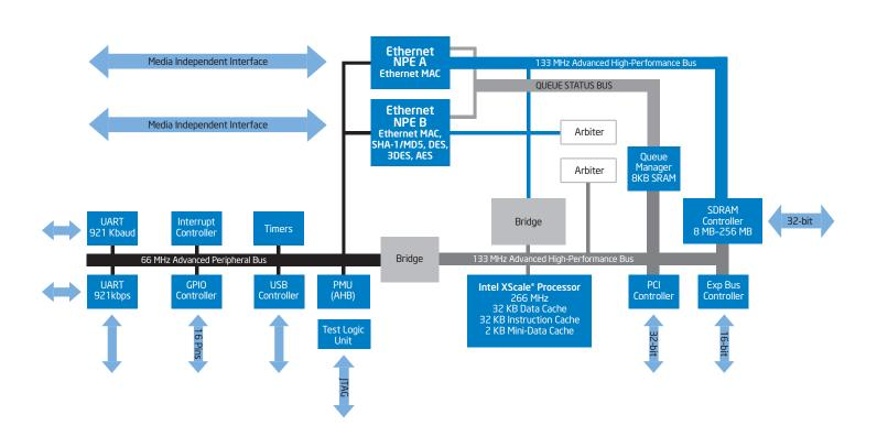
network processor. This provides maximum flexibility for all interfaces, especially when dealing with security issues over wireless. This high-performance architecture can support bulk encryption/decryption rates of up to 70 Mbps for DES, 3DES and AES algorithms.
