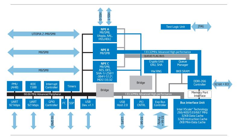
Figure 1: Intel® IXP465 Network Processor
