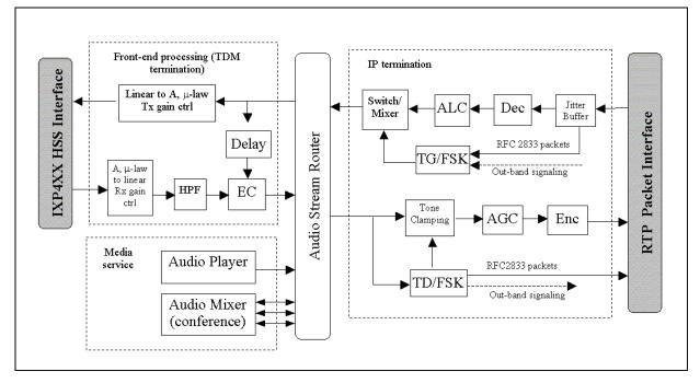
The voice sample block, after its signal level is properly adjusted by the Automatic Gain Control module (AGC), is next processed by the voice Encoder to generate audio data packet to be sent through the IP stack. The encode type is selectable, and determines the compression rate on the compressed voice.
