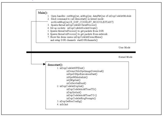
In Kernel mode, function demostart() first calls ixDspCodeletNPEInit() to initialize NPE. ixDspCodeletNPEInit() will downloads the NPE code to NPE-A using function ixDemoUtilsNpeImageDownload(), start the NPE-A execution using ixNpeDlNpeExecutionStart(), initialize the message component using ixNpeMhInitialize(), and initialize the QMgr component using ixQMgrInit() and ixOsServIntBind() if ixp425\_eth.o is not going to be used.
