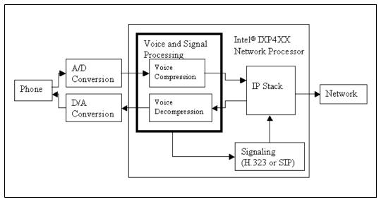
DSP software is a software module that provides the basic voice and signal processing functionalities as highlighted with a bold frame in Figure 1. It does not cover other functions such as signaling.
