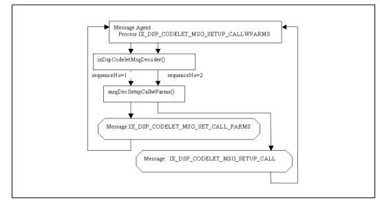
Now the Message Agent finishes processing the user-defined message IX\_DSP\_CODELET\_MSG\_SETUP\_CALLWPARMS. But it now has two new user-defined messages waiting for processing, which are created during processing the message IX\_DSP\_CODELET\_MSG\_SETUP\_CALLWPARMS.
