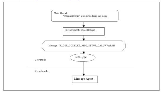
Because the resource type field in the message header is Message Agent XMPR\_MA, the DSP software module will direct the message of type IX\_DSP\_CODELET\_MSG\_SETUP\_CALLWPARMS above to the Message Agent.
