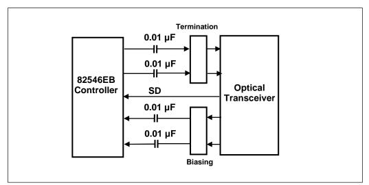
82546EB fiber-based applications will use the SERDES interface to drive a 1000BASE-SX or 1000BASE-LX optical transceiver as illustrated in the following figure. The 82546EB controller is internally terminated, so no external termination is required.
