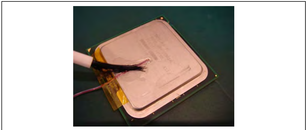
Figure 7-34. Application of Accelerant
