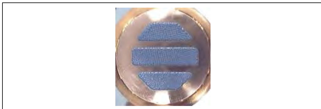
Figure 6-3. Bottom View of Copper Core Applied by TC-1996 Grease
