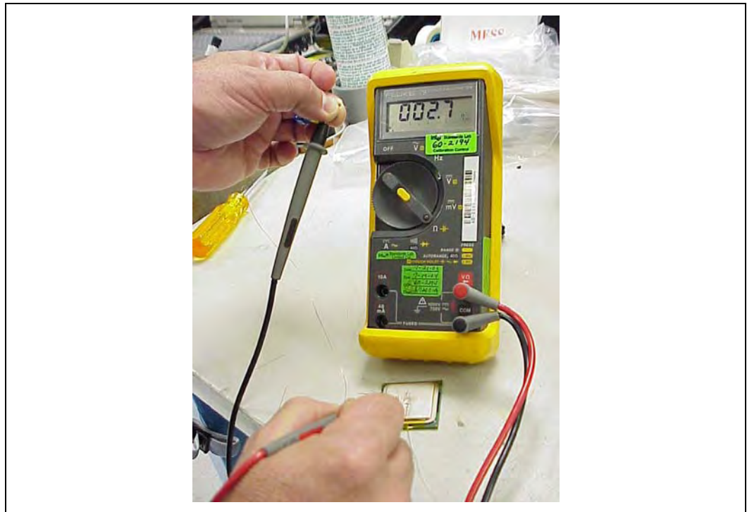
Figure 7-23. Measuring Resistance Between Thermocouple and IHS
