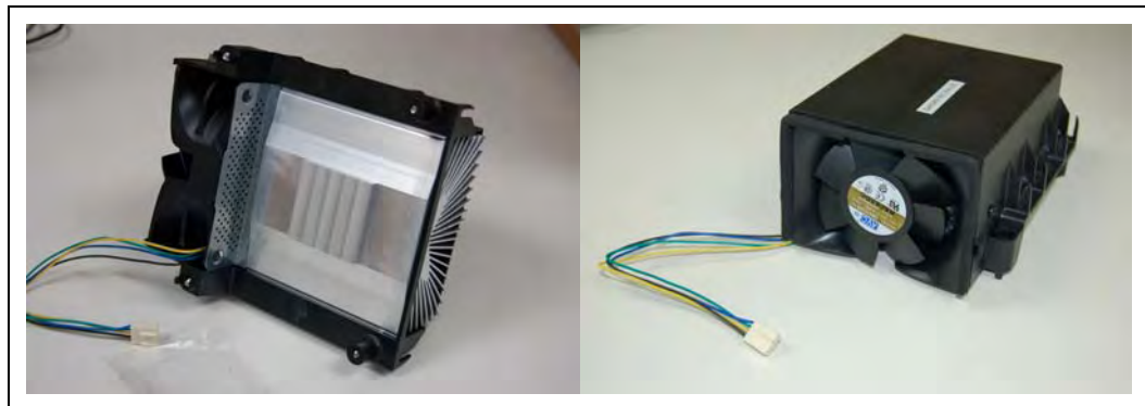
Figure 5-4. Intel Type II TMA 65W Reference Design
