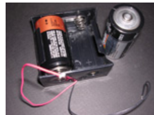
"D" size batteries and holder
