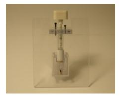
The next step is figuring out how the parts of the dispenser will work. In this case, a model was made of the mechanical component, the soap-dispensing mechanism. With this model, engineers can trial and test how the mechanism will work.
