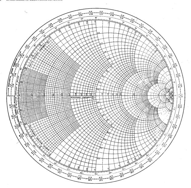
FIGURE 13.10 A photographic reduction of one version of a useful Smith chart (courtesy of the Emeloid Company, Hillside, N.J.). For accurate work, larger charts are available wherever fine technical books are sold.
