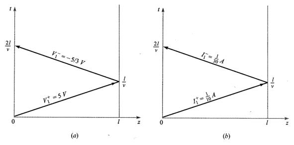
FIGURE 13.20 Voltage (a) and current (b) reflection diagrams for Example 13.5.
