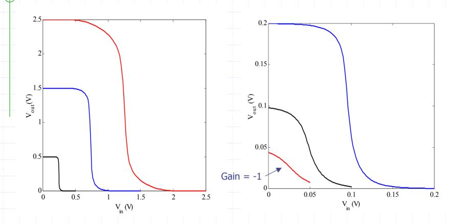
The gain can be improved by lowering the supply voltage, however, below a few tenths of a volt, the gain deteriorates.
