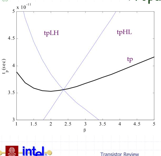
The smallest delay is for  $\beta$ =1.9. Equal propagation delays require  $\beta$ =2.4.
