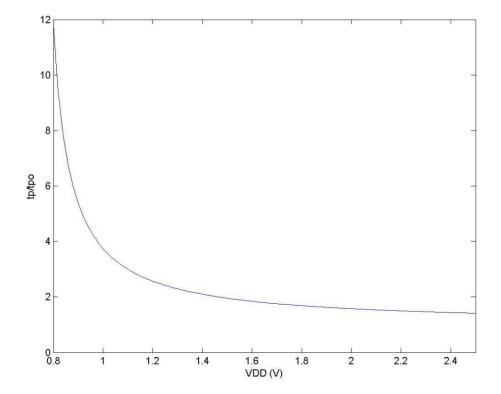
Note that supply voltages below 1.1 V cause an enormous increase in the propagation delay.
