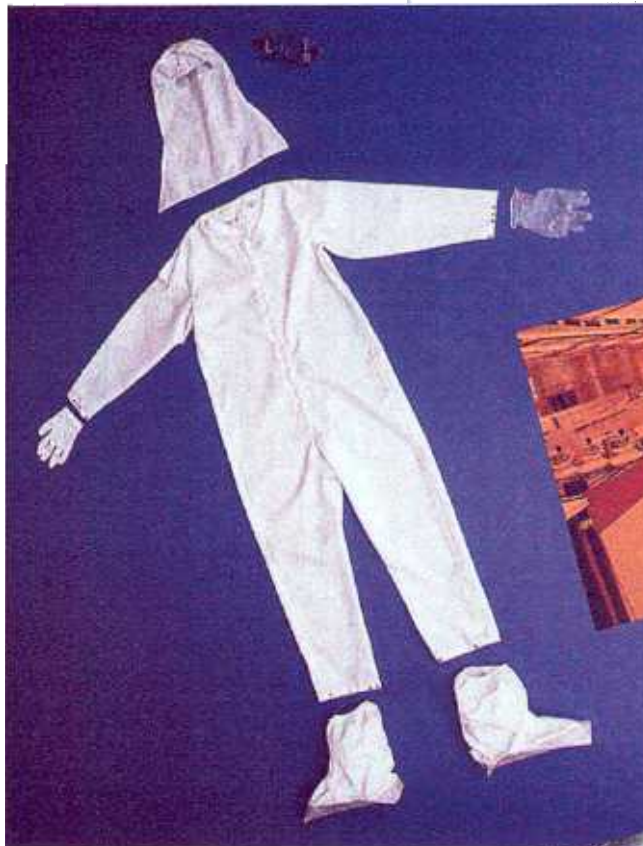
"Bunny" suits were introduced at Intel in 1973 with the opening of Fab 3 in Livermore. Pictured here are the pieces of the typical clean room garb worn today.
