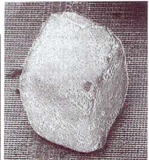
Scanning Electron Microscopic view of a common table salt crystal resting on Intel's high-density 27128 EPROM. Each of the 27128's 131,672 cells measures approximately 7 microns (7 millionths of a meter) across, in contrast to the average salt crystal's 300 microns.
