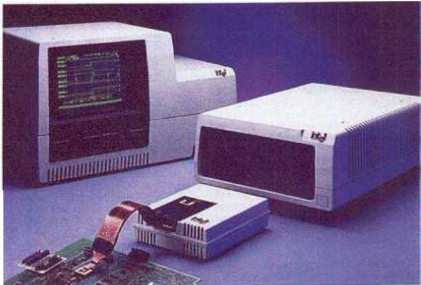
One of Intel's newest design tools, iICE (Integrated Instrumentation and In-Circuit Emulator) brings together high-level language software debugging, logic analysis, and in-circuit emulation in a
