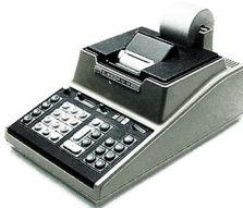
This calculator from Japanese manufacturer Busicom was the first microprocessor application.
