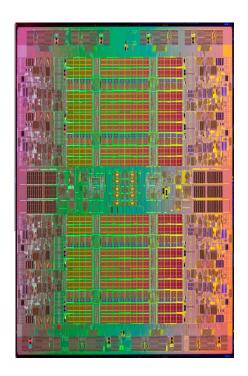
**Intel Itanium processor 9500 series die.** 8 cores, 32MB Last Level Cache, and over 3.1 Billion transtors.
