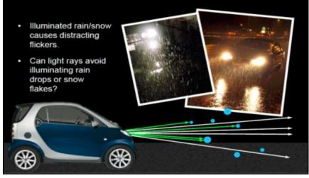
The smart headlight can detect and track rain drops as they fall, and then selectively 'turn off' light rays at the predicted future rain drop locations. Risk is minimized and driver's visibility is maintained.
