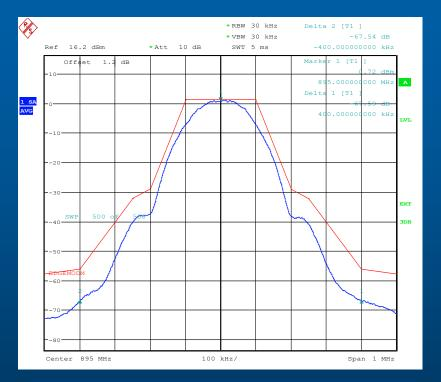
EDGE (without pre-distortion) Power = +8,5dBmEVM = 1,46%Noise in GPS Band = -166dBc/Hz
