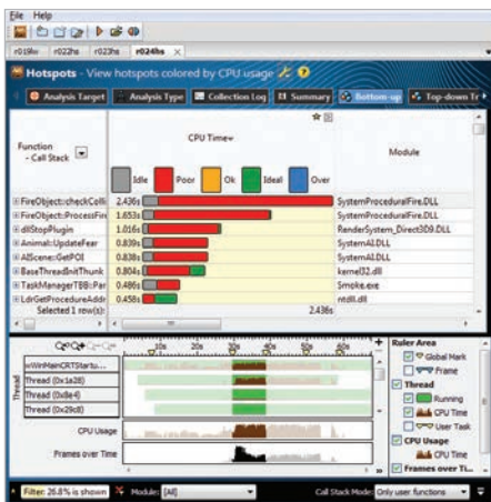
Intel® VTune™ Amplifier XE Performance Profiler helps developers tune single-node threading by visualizing thread behavior, evaluating thread load balancing, and finding thread synchronization bottlenecks.
