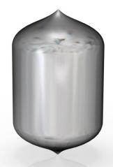
Monocrystalline Silicon Ingot – scale: wafer level (~300mm / 12 inch) The ingot has a diameter of 300mm and weighs about 100 kg.
