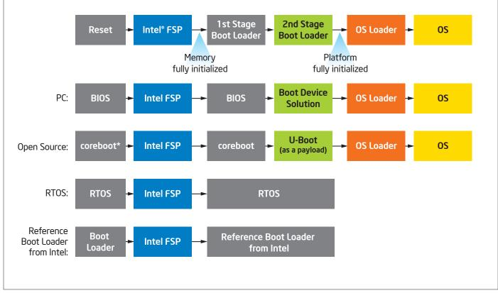
Figure 2. Boot Solutions with Intel® Firmware Support Package
