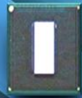
DISCRETE FCMB <1 mm thick
