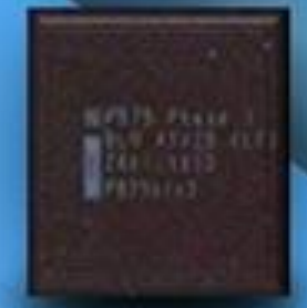
SINGLE DIE FCBGA 1.6mm thick
