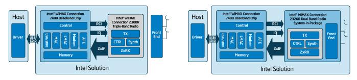
OEMs may choose to integrate the Intel WiMAX Connection 2400 baseband chip with either a stand-alone radio chip (left) or the SIP radio module (right).
